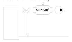
For Air outlet through an Air vent (not supplied from the factory) is on top of **NONAIR**®, depending on the size, 1 to 3 pcs of 1/2" female threaded sockets. For future service of the Air vent mount a 1/2" ball valve (male thread in/female thread out) in between. If the Air vent has 3/8" inlet mount the 1/2 x 3/8" reduction supplied between the ball valve and the Air vent.
